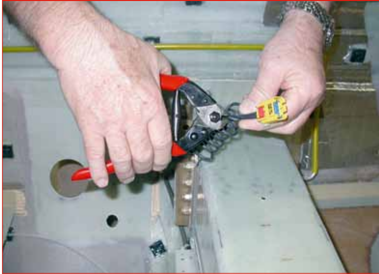
Picture 34: Third method to cut the cable connecting the electrical module assembly to the inflator assembly
