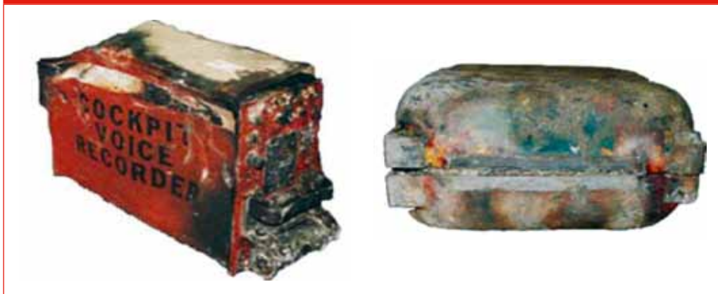
Picture 6 and 7: Damaged flight recorders
