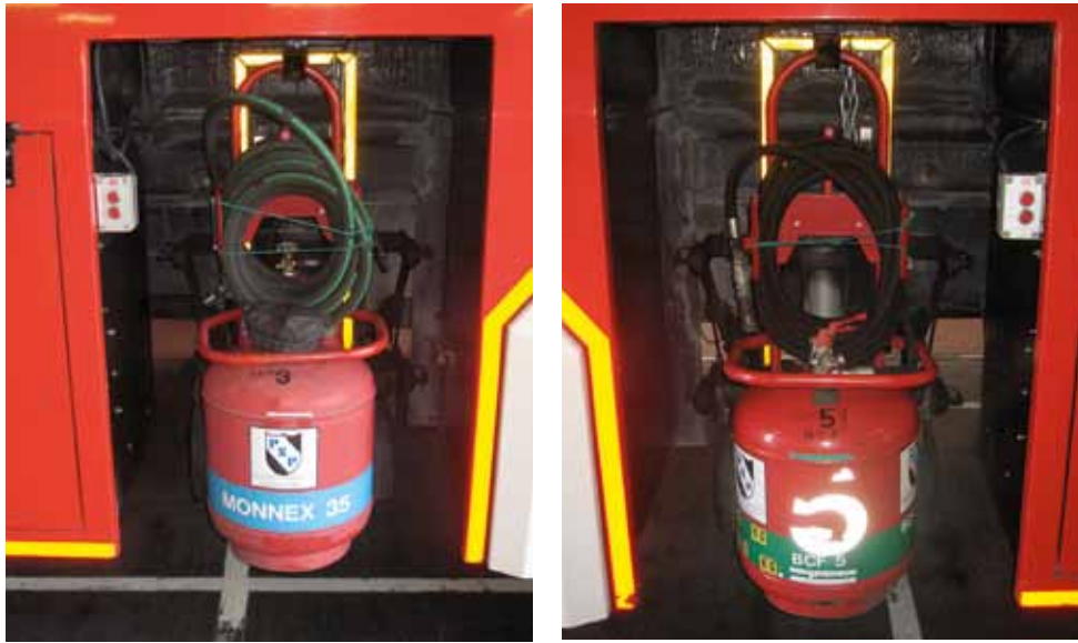
Pictures 4 and 5: Rescue and Fire Fighting Service supplementary firefighting media, bulk dry powder (Monnex) and bulk BCF mounted on a trolley assembly
