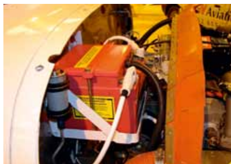
Pictures 7 and 8: Location of battery in general aviation aircraft
