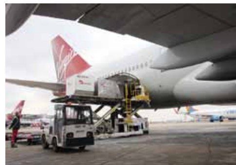
Pictures 3 and 4: Example of typical cargo bay door (top hinged)
