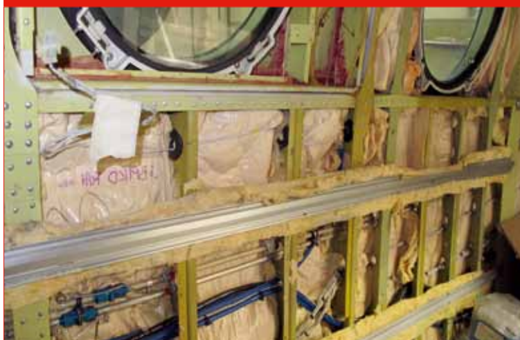
Picture 5: Internal fuselage construction of a small passenger carrying aircraft with a pressurised cabin
