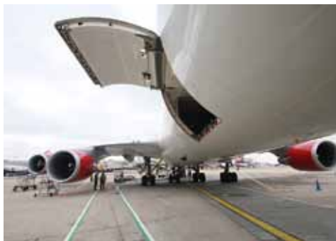
Pictures 3 and 4: Example of typical cargo bay door (top hinged)
